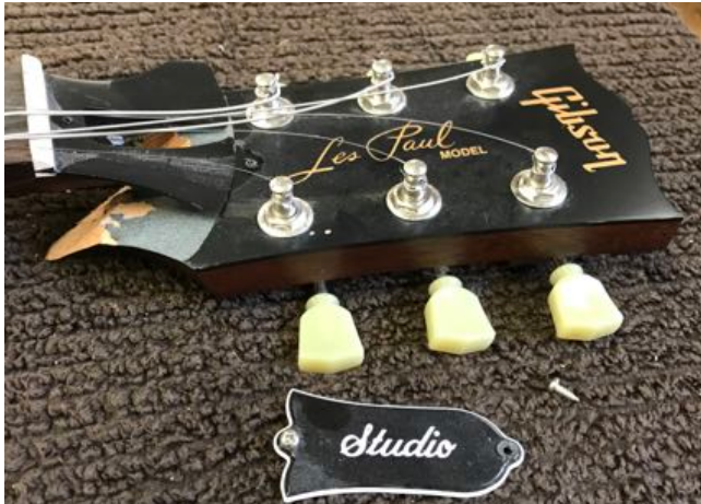
The damage (“clean” primary break plus a nearly-invisible hair-line crack)
