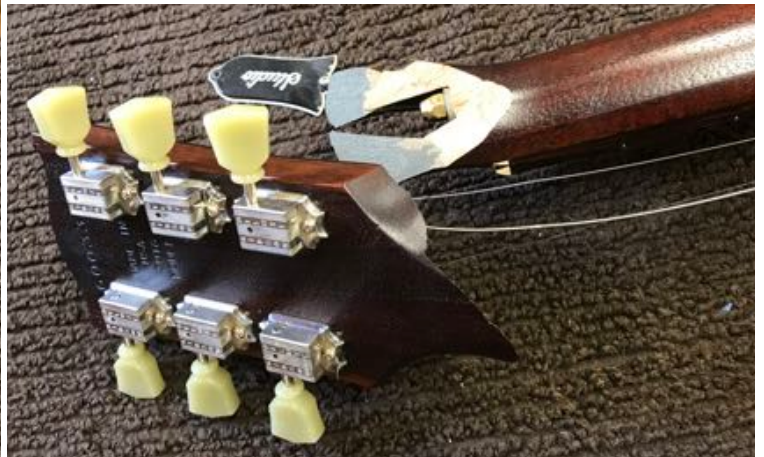
The damage (“clean” primary break plus a nearly-invisible hair-line crack)
